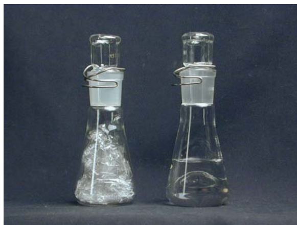
Figure 4 Left bottle: JunFunori film not yet ground, right bottle: JunFunori solution.
