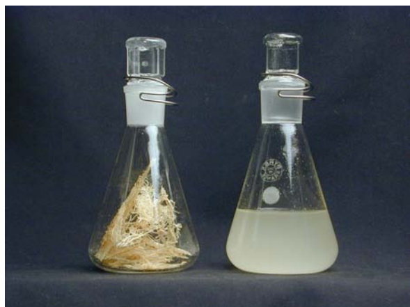
Figure 3 Left bottle: dry funori , right bottle: extracted funori solution.
