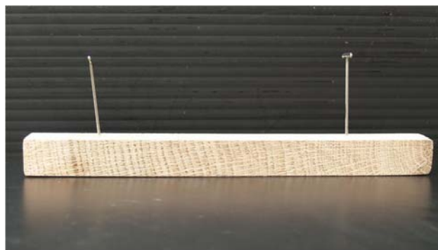
Figure 3. Sample of white oak with measuring pins.
