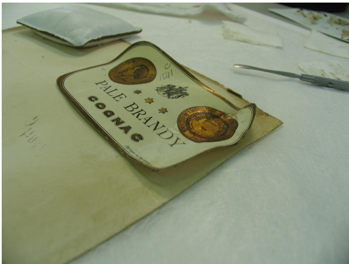
Figure 1: Printed label adhered to scrapbook page. Adhesive is water-soluble except in areas immediately adjacent to gold-coloured ink.
