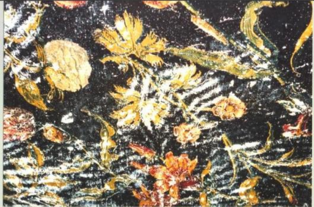
Figure 4: Residue from the adhesive on the reverse after removal of the backing (BK-KOG-41).
