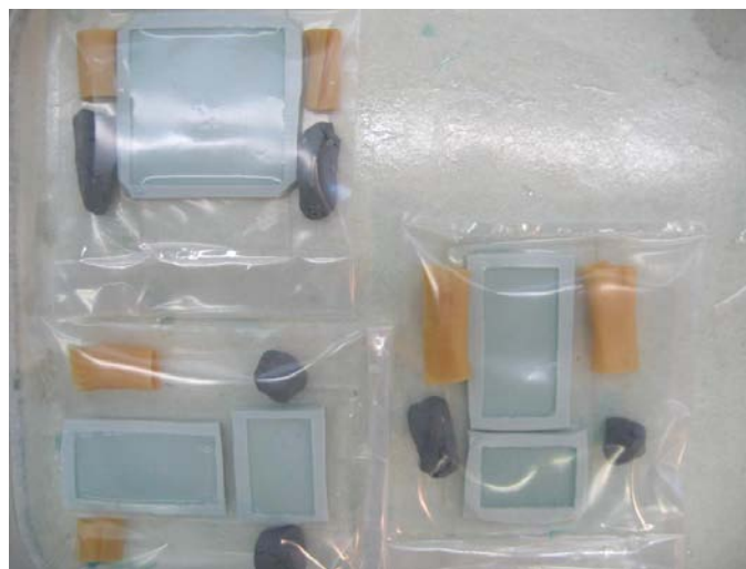
Figure 2: open-faced silicone moulds in polyethylene bags
