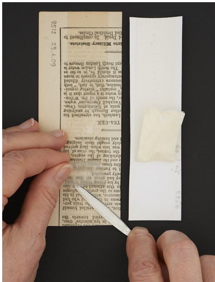
Figure 3. Mechanical removal of tapes from Punch paper and RC paper.
